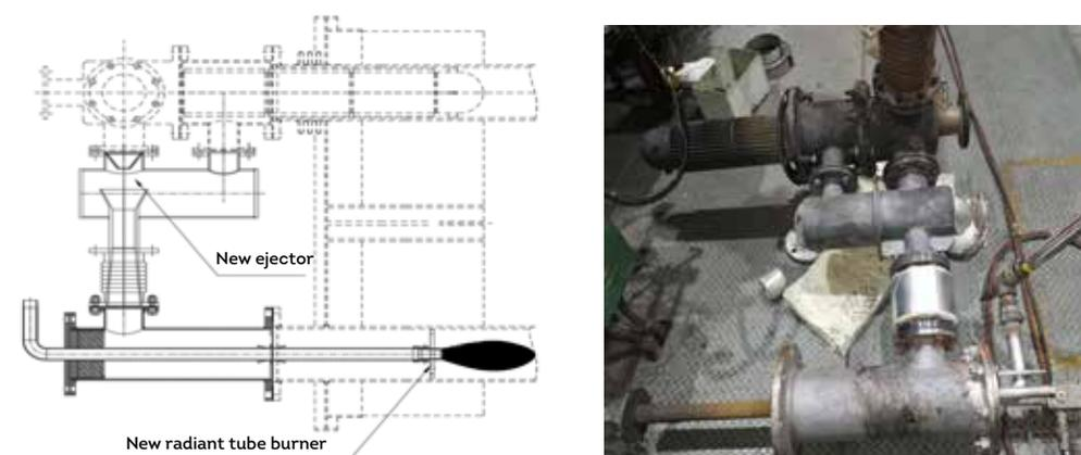
**Fig.2.4** Structure diagram and photo of the new radiant tube burner and ejector
