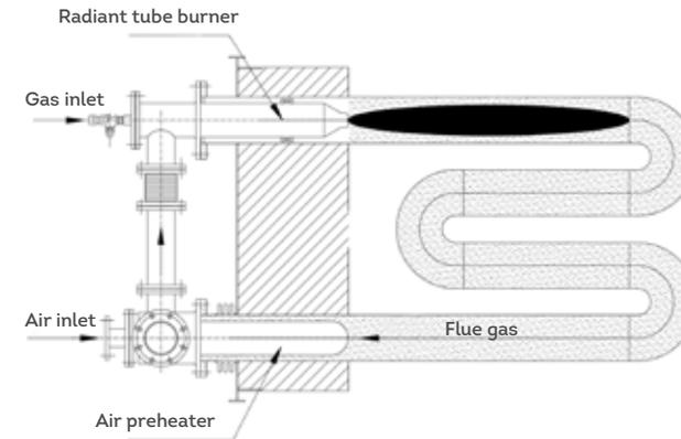
**Fig.2.1** Installation diagram of the radiant tube burner and heat exchanger
