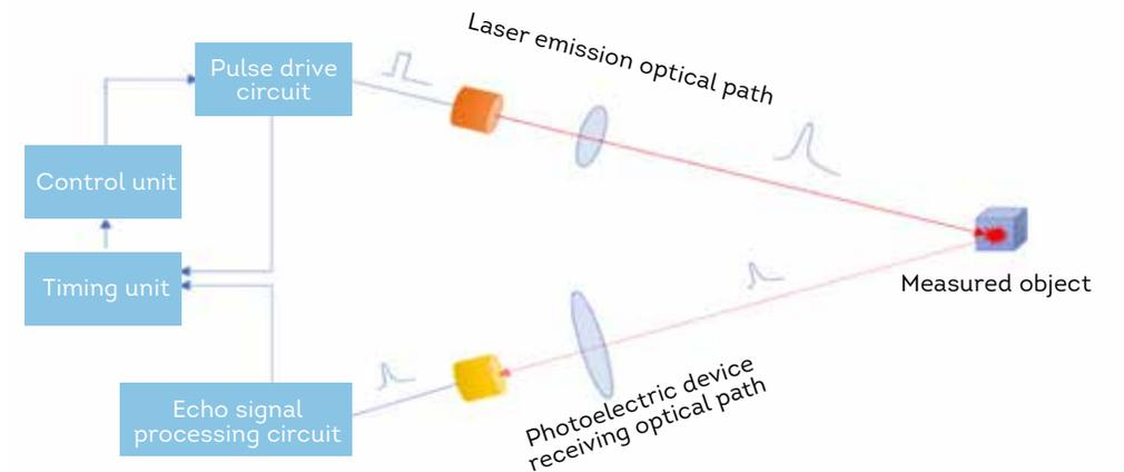
Fig.3 Fundamental diagram of TOF camera
