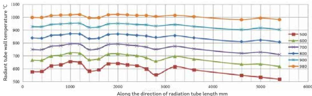
**Fig.2.6** Surface temperature curves of the radiant tube at different furnace temperatures
