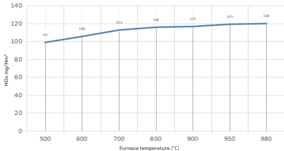
**Fig.2.5** NOx concentration curve of the burner at different furnace temperatures
