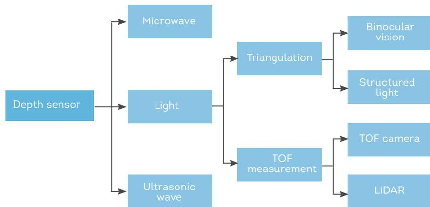
Fig.2 Depth sensor classification<sup>[5]</sup>
