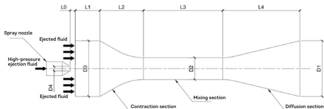
**Fig.2.3** Structural schematic diagram of ejector
