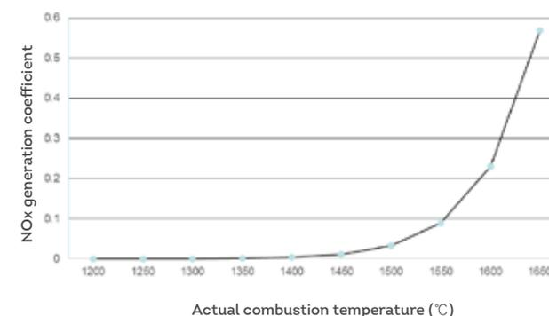
**Fig. 1.1** Relationship graph between thermal NOx production and actual combustion temperature
