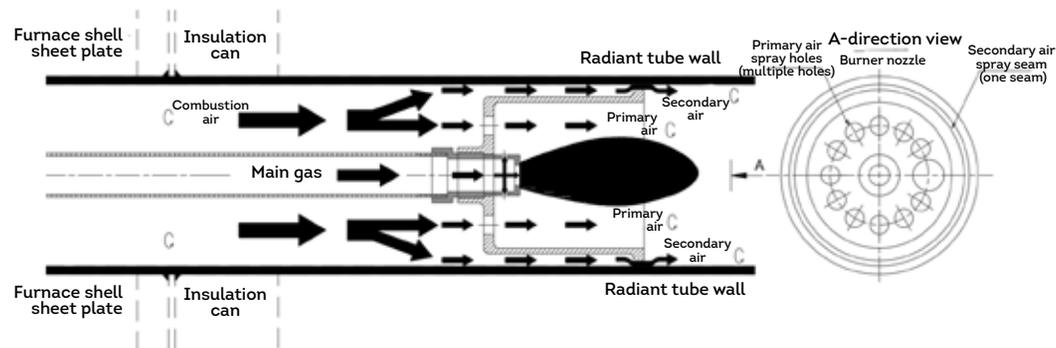
**Fig.2.2** Schematic diagram of staged combustion of air
