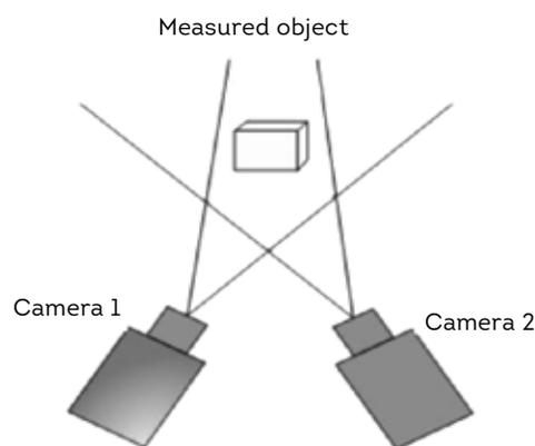
**Fig.5** Fundamental diagram of binocular visual ranging
