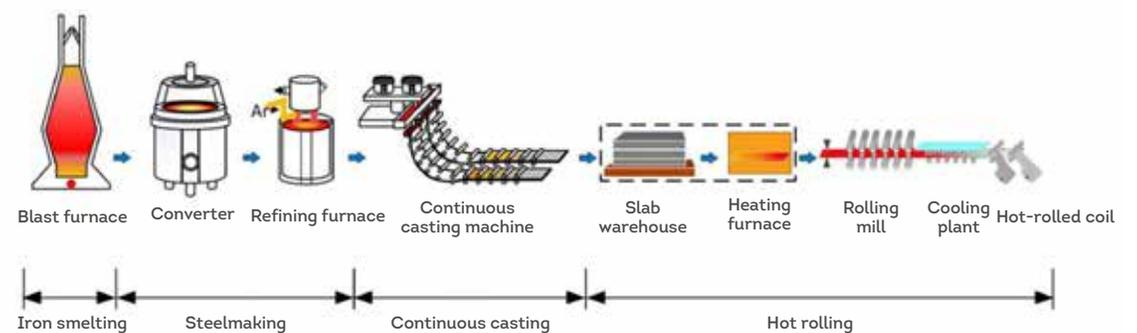
Fig.1 Long-process steelmaking process
