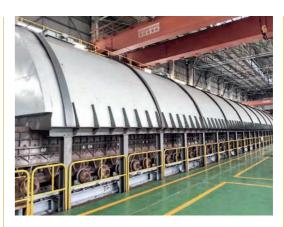
The flue gas circulation systems for three sintering machines have all been put into operation, each with effective ventilation area of 500m<sup>2</sup>
