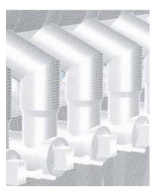
Structural grid used in travelling grate model
