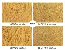
Comparison of crystal grains in the FWD and CFMC
