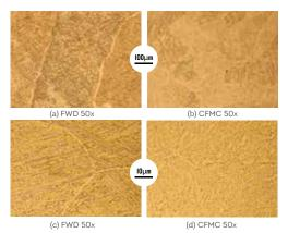
Comparison of crystalline phases of nickel-based superalloy specimens produced by FWD & CFMC fig.9
