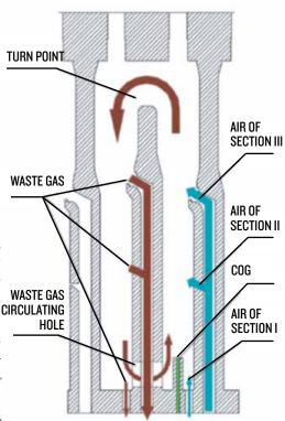
Schematic diagram of section-wise heating and waste gas circulation
