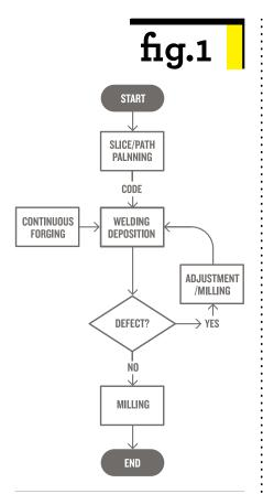
Flow chart of CFMC additive manufacturing
